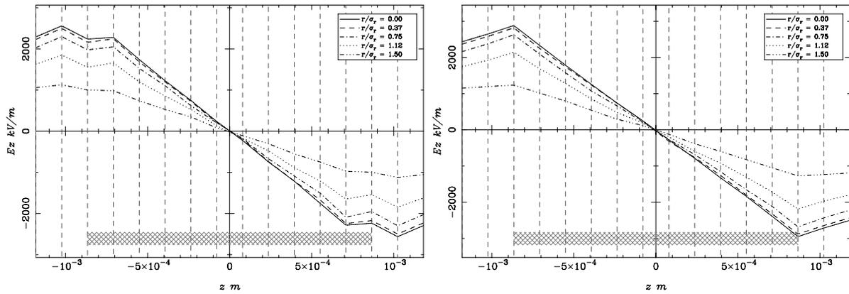
Figure 3: Longitudinal electric field of a short bunch with aspect ratio 2:  $E_z$  along the  $z$ -axis calculated with FFT (left) and MG (right).
