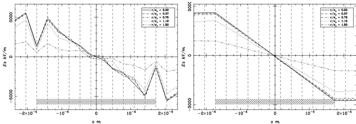
Figure 4: Longitudinal electric field of a short bunch with aspect ratio 10:  $E_z$  along the  $z$ -axis calculated with FFT (left) and MG (right).
