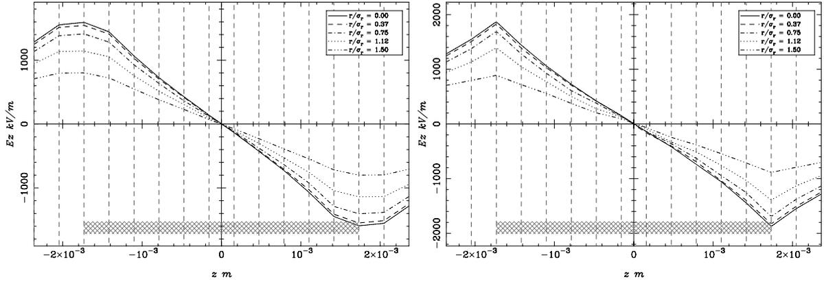
Figure 1: Longitudinal electric field of a bunch with aspect ratio 1:  $E_z$  along the  $z$ -axis calculated with FFT (left) and MG (right).
