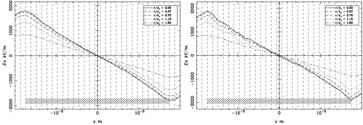
Figure 2: Longitudinal electric field of a bunch with aspect ratio 1:  $E_z$  along the  $z$ -axis calculated with FFT (left) and MG (right).
