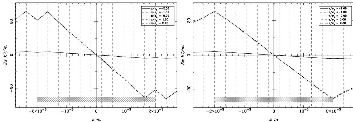
Figure 5: Transverse electric field of a long bunch with aspect ratio 0.01:  $E_x$  along the  $x$ -axis calculated with FFT (left) and MG (right).
