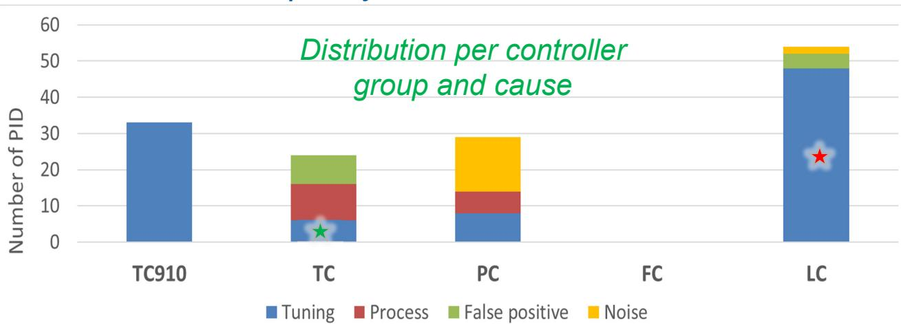
Distribution per cryogenic system & controller group
