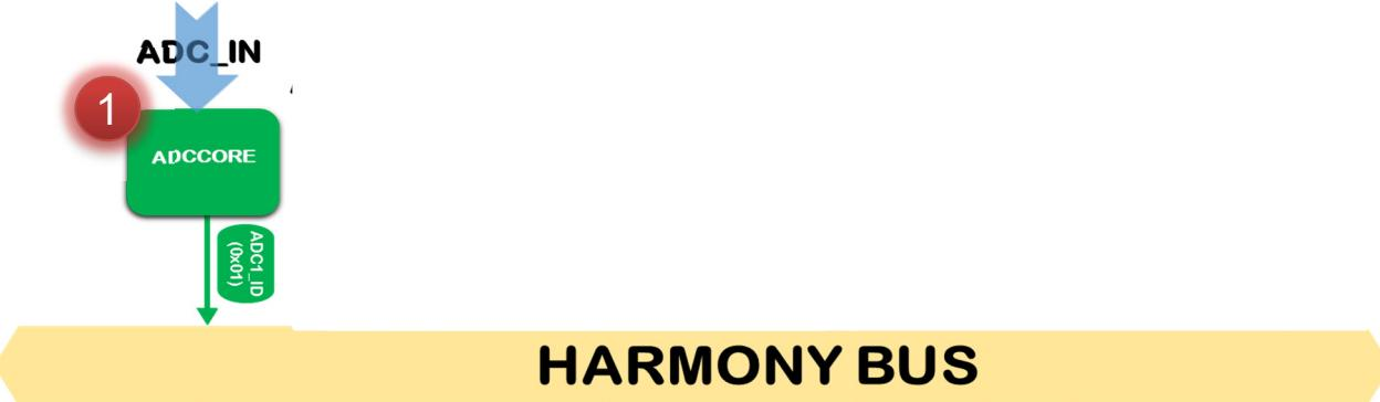
1 Data acquired by the ADC, is read by the ADCCORE block (ADC1\_ID).
