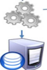
The new MERGE SERVICE aggregates the output of both CMT and SST and writes the resulting XML experiment definition to the database.
