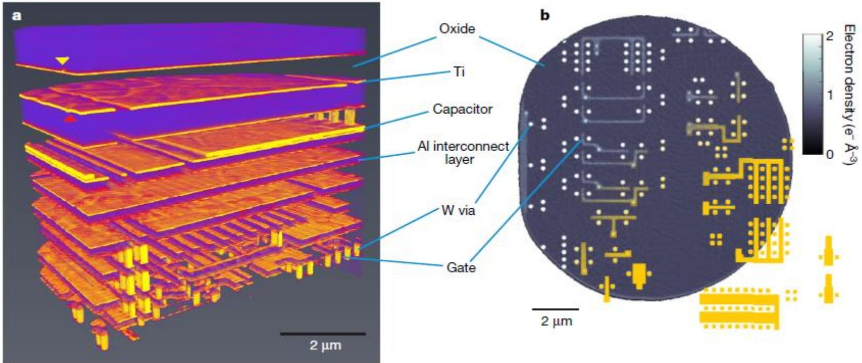
Fraction of the chip selected: set-reset memory latch
