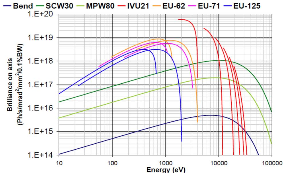
Tuning ID magnetic field and orientation, and playing with beamline optical elements large range of photon energy and polarization are available
