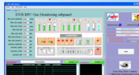
RPC GAS Monitoring GUI
