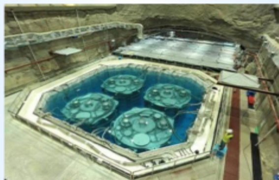
Muon Water Pool, RPC & 4 ADs in Far Hall
