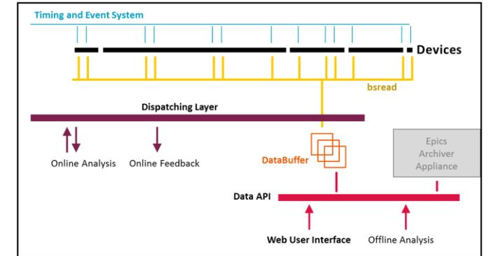
Beam Synchronous Data Acquisition System
