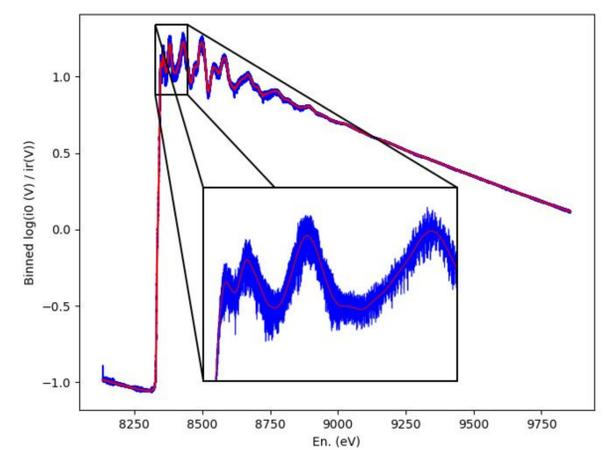
The binning is done using a Gaussian Filter, by a convolution of the original data and a Gaussian function.
