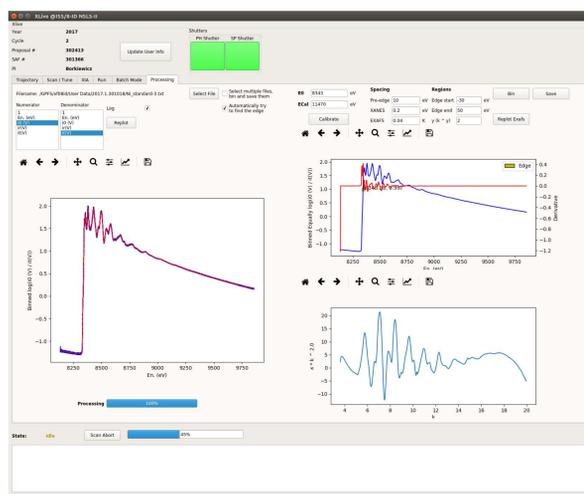
After running the scans, the last step is opening the data, binning and exporting it. The last tab of the software, "Processing", is used for that. The exported file typically has around a thousand points after binning – typical number for spectroscopy measurements.
