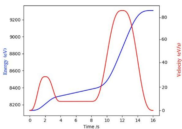
Double Sine/Constant Edge trajectory: The user defines the first, last and edge positions (eV), pre-edge and post-edge durations (s) and the edge velocity. The monochromator will follow this trajectory when the user is running scans.
