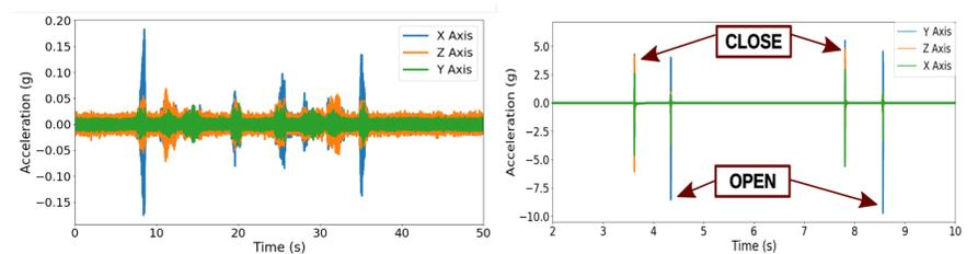
Figure 4: Sample vibration when robot is moving (left) and on gripper open/close (right).
