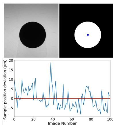
Figure 3: Sample Projection (top, left) and binarized image (top, right) and X-axis position deviation (bottom).
