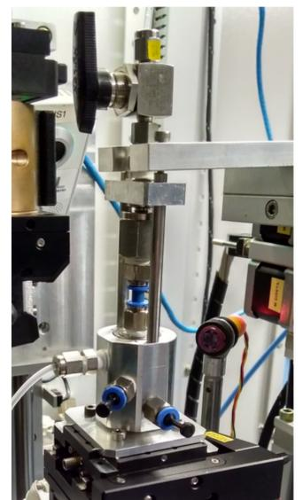
Figure 5: Flux cell mounted under IMX rotational stage.
