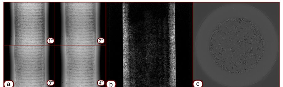
Figure 6: Sample projections during injection (a), first and last projection subtraction (b) and dry sample tomography slice (c).
