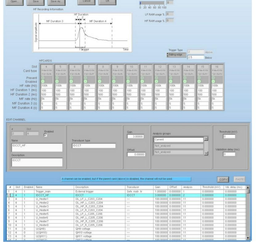
When the acquisition is started, the signals are stored in circular buffers, according to the selected duration D1 for HF/MF and LF. Once a quench is detected by the dedicated quench detection system, the recording of
