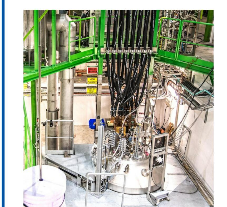
. Useful length 5000 mm / diameter 800 mm • Working temperature 1.9 - 4.2 K Vertical arrangement
