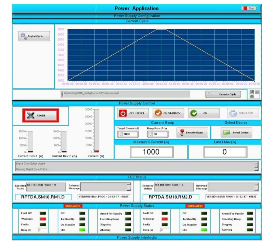
application *POWER* synchronously the two 15 kA power converters from the control room. All the status information from the Function Generator Controllers, version 2.00 (FGC2) and from the high power stages are presented to the operator.
