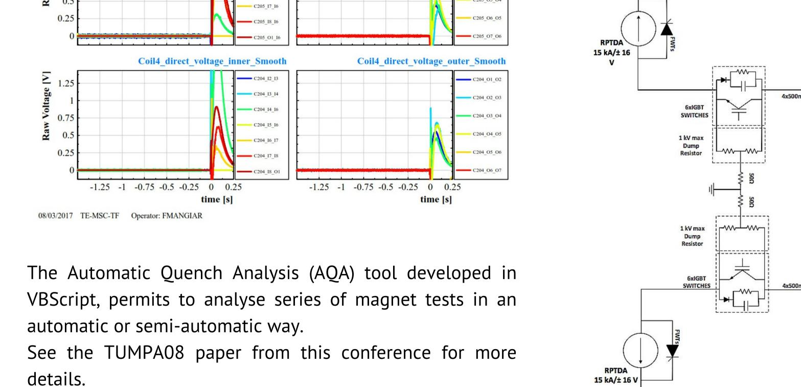
The need for a test bench to evaluate a new generation of superconducting magnets in the framework of the HL-LHC project initiated several R&D activities. We handled those related to the data acquisition system and to the remote control of two 15 kA power converters. After a survey, the PXIe platform has been selected for the DAQ system and a dedicated application has been developed in LabVIEW™.
