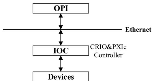
The control System structure is based on EPICS.
