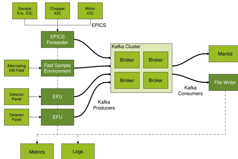
System architecture and data flow. The components in dark are being developed as part of the pipeline; dashed lines represent metrics and log messages.
