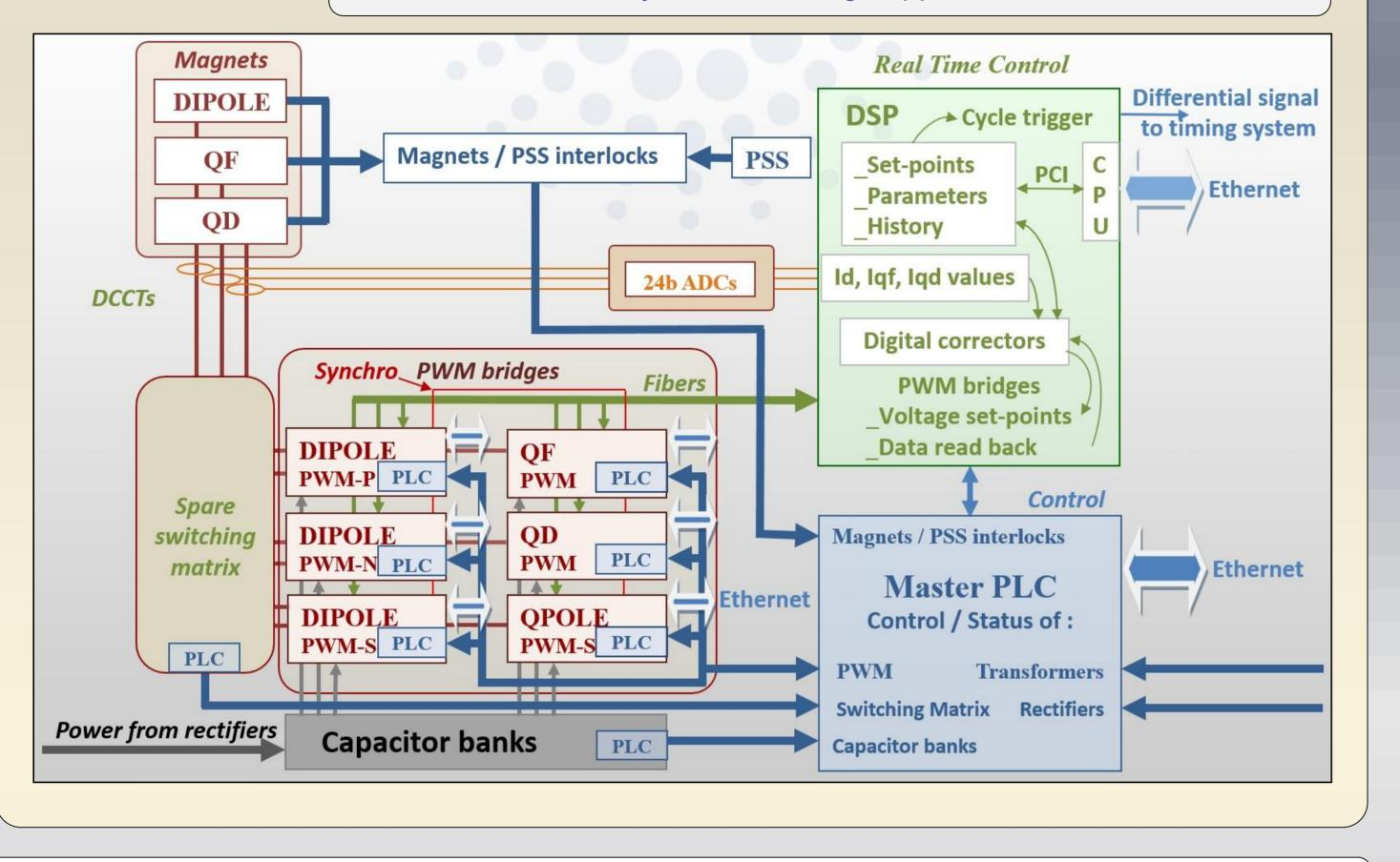
All pieces of equipment are equipped with a dedicated PLC connected to a server through Ethernet. These PLCs are controlling the states of the different units and reporting to a master PLC itself controlled by a remote Tango application. All commands and safety aspects are managed by the master PLC while the history of events goes directly from each PLC to the Tango server.
