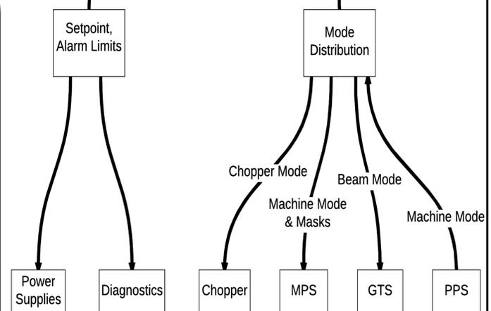
Figure 4: Data flow between RPS and sub-systems
