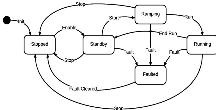
Figure 3: RPS finite state machine model
