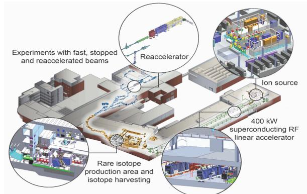
Figure 1: Layout and major components of FRIB
