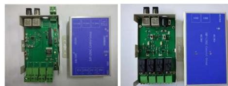
Fig.4 Left: The photoelectric conversion module on the device side is mainly used to interconnect the signal between the low level equipment and the front-end FPGA controller.
