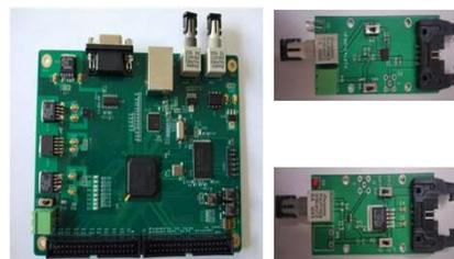
Fig. 3 Front-end FPGA control board and optical signal transceiver module.
