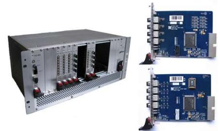
Fig. 5 MIS crate and function module
