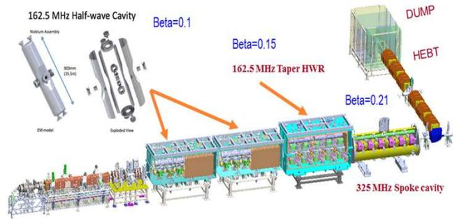
Fig. 1 The Injector II proton linear accelerator
