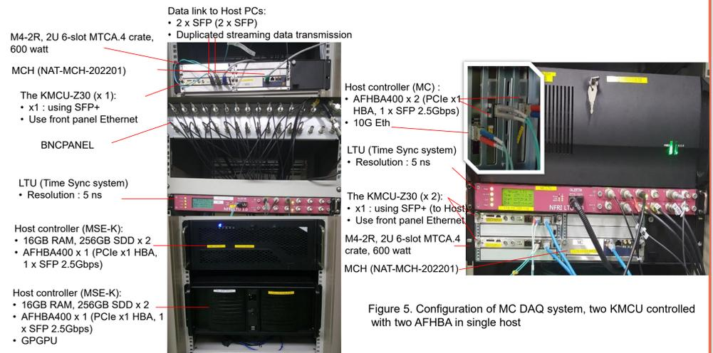
Figure 4. Configuration of MSE-K DAQ system, duplicated streaming data transmission from single digitizer to two systems (can do three way streaming data transmission with PCIe-uplink)
