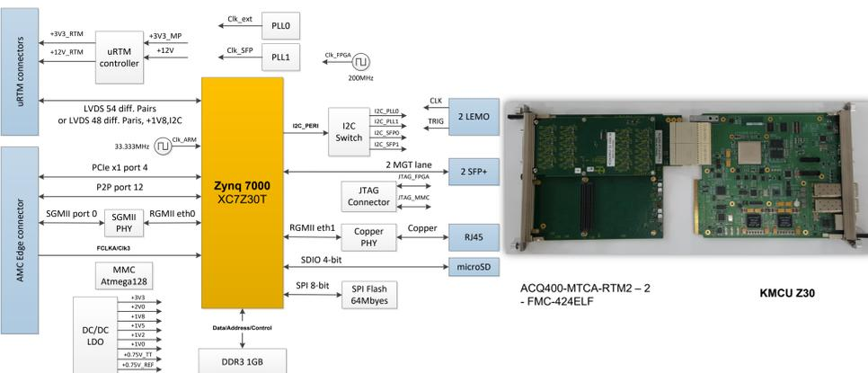
Figure 1. A Block diagram of KMCU-Z30 ( changed FPGA, 2 SFP front interface and Backplane (PCIe x4 -> PCIe x1 Gen2) and KMCU-Z30 & ACQ400-MTCA-RTM2 with digitizer [3]
