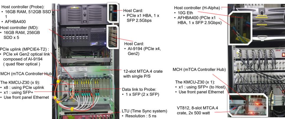
Figure 2. Configuration of MD (with PCIe uplink) & Probe DAQ system in single create
