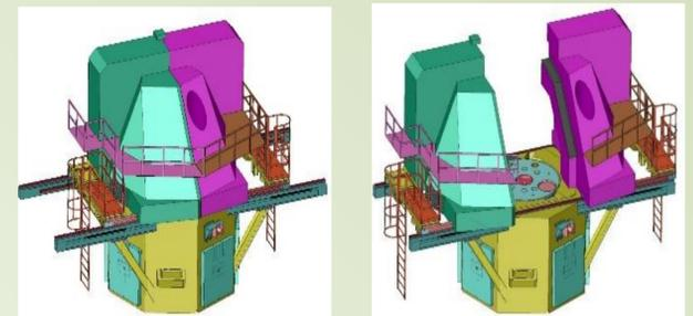
Figure 1: Layout of the NSC KIPT Neutron Source biological shielding
