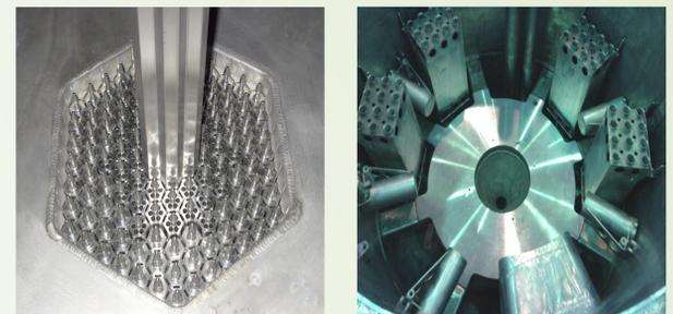
Figure 2: NSC KIPT neutron source core with target
