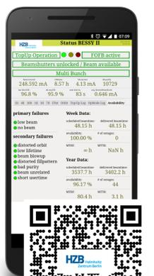
Availability of synchrotron radiation as percentage of "promised" scheduled beamtime as well as MTBF and MTTR are calculated on a per week and per year basis. Overall performance is visible in unambiguous figures. Same metric has been back-calculated for better comparison.
