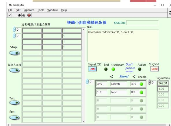
The Short Message Service (SMS) information is still necessary to send to relative staffs from sub-system event. Especially, the WIFI of mobile phone is turned off. This toolkit GUI is developed by labview tool. It can be also compatible with EPICS and TLS original control system.
