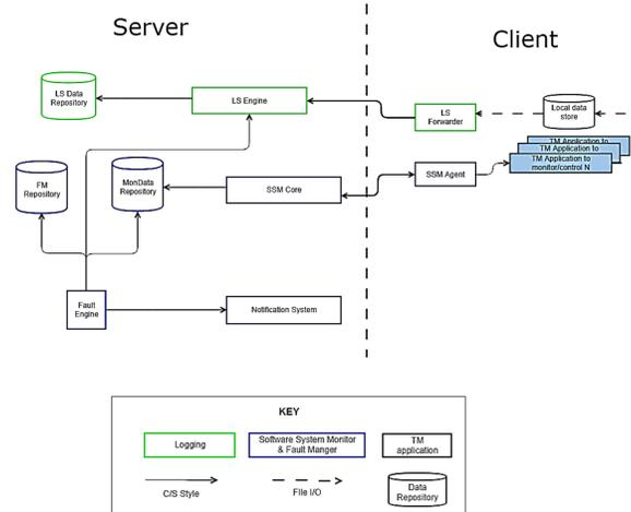
Figure 2: the architecture of SSM and Fault Manager. AI Algorithms are implemented in the Fault Engine Module
