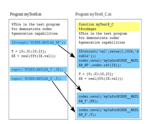
>Creating myTest8\_C.m based on myTest8.m for further MATLAB codegen processing >Inserting function name myTest8 C >Inserting %#codegen directive
