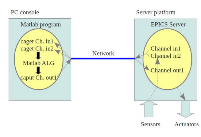
MATLAB programs at PSI are mostly used in closed loop control applications as illustrated on the left.
