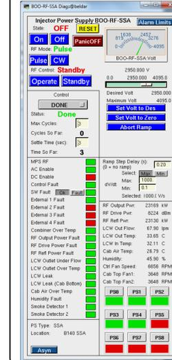
SSA control via the MODBUS-based XPORT device. EPICS Soft IOC SSA runs on Linux Server:
