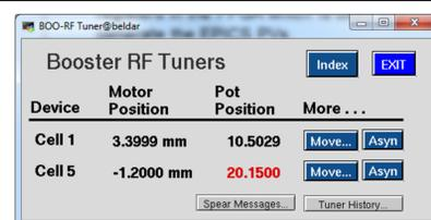
Tuner control via EtherCAT based Beckhoff modules in a driver chassis that controls two stepper motor-controlled tuners in cell1 and 5 of the 5-cell Booster RF cavity. EPICS Soft IOC MC runs on LinuxRT Server:
