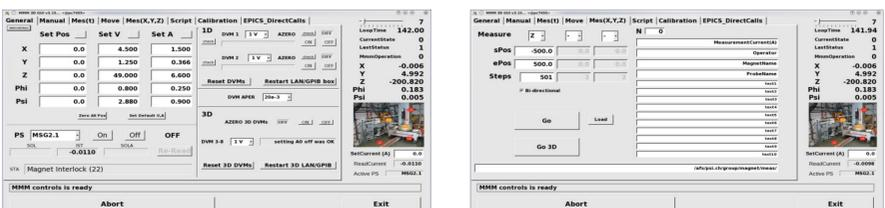
The MMM state machine software is developed by magnet measurement and control system experts, which makes it highly optimized and extremely efficient for all MMM operations. The MMM client and server programs communicate via EPICS. They both are combined into the Hall probe process control application, which can handle a variety of basic operational modes.
