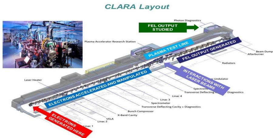
By adding a laser, the transverse field of the radiation will interact with the electron beam causing micro-bunching of the electrons. The micro-bunching causes the free electron laser, FEL, to generate short, highly stable, coherent radiation pulses that are several orders of magnitude greater than the undulator..
