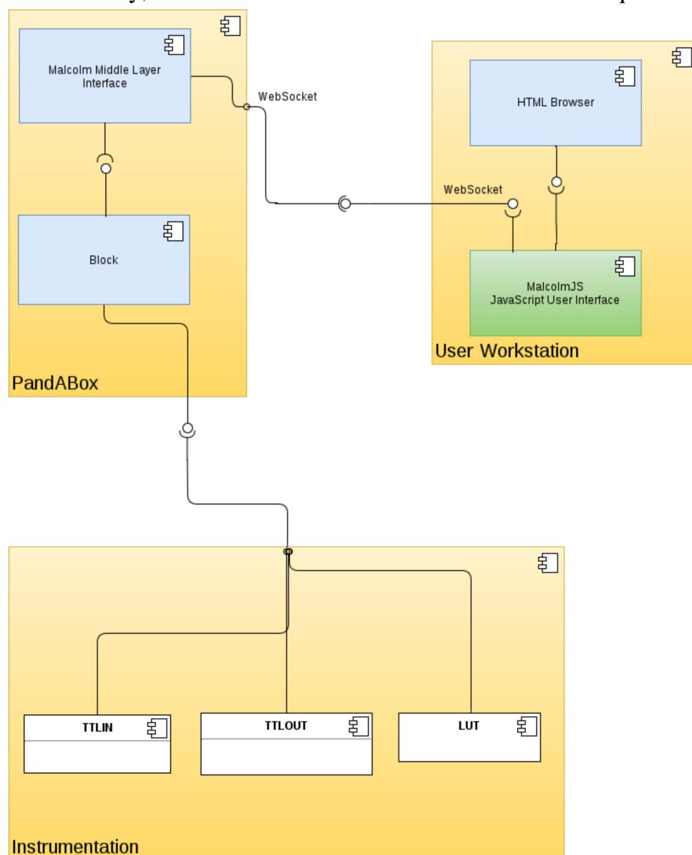
Websocket communications expose the structure of Malcolm Blocks via a JSON protocol over websockets. There is a client MalcolmJS library that is used to create a web GUI to allow configuration/load/save of Blocks from a web browser, like in a PandABox.
