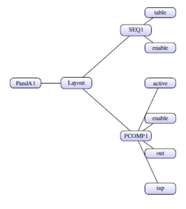
MalcolmJS must, therefore interrogate the attached device(s) for information on all the available function blocks, attributes and associated meta-data. The collection of internal resources then being listed in a "palette" in the right hand side-pane.
