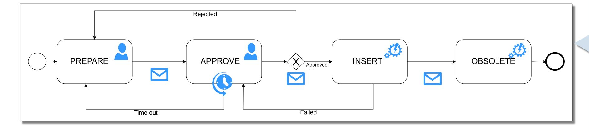
DIP Contract Monitoring relies on a simple workflow that backs the application's front-end user interface through the same aforementioned three basic stages: registration, approval, and insertion into a C2MON configuration database.
