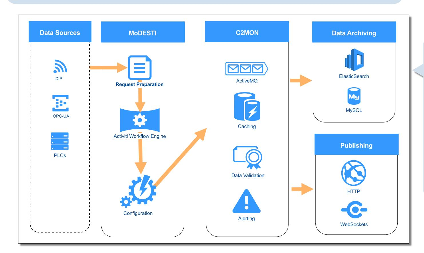
To address different use cases, MoDESTI supports modular plug-ins. Each MoDESTI plug-in contains a schema describing the data domain and its constraints, and also provides a Business Process Model and Notation (BPMN) workflow specification.
