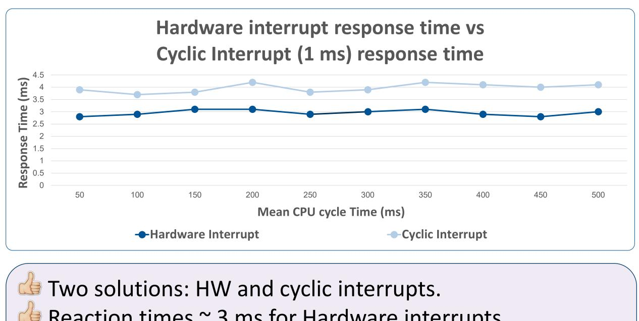
Reaction times ~ 3 ms for Hardware interrupts.
