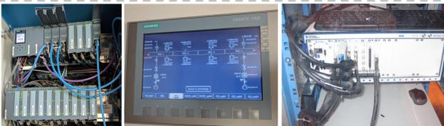
Figure 8: Vacuum Control (left), slow control touchscreen (middle), beam diagnostics (right).
