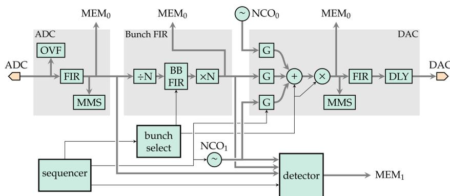
This figure shows the data processing for a single LMBF/TMBF channel:
