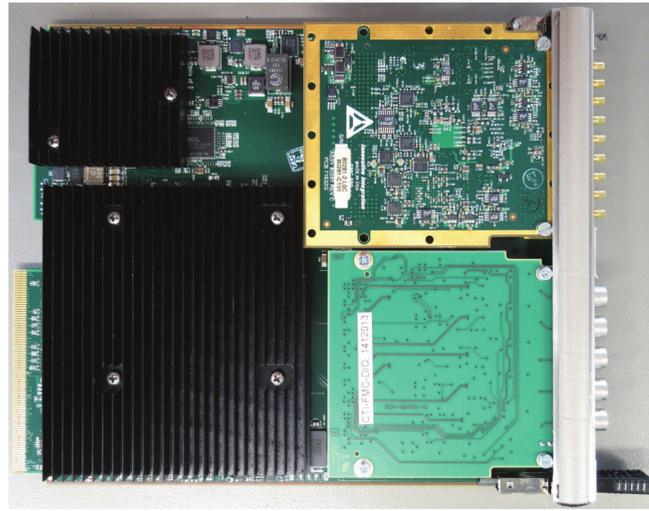
Here we see the chosen hardware platform, with a 500 MSPS ADC/DAC FMC card at top right, and a Virtex-7 690 FPGA under the heatsink at bottom left.
