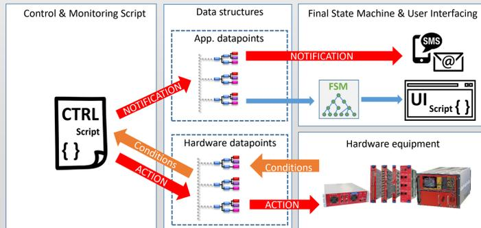
Figure 1: Simplification of the Preshower DCS architecture
