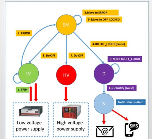
Figure 2: Internal FSM representation for a CMS ECAL supermodule (SM)
