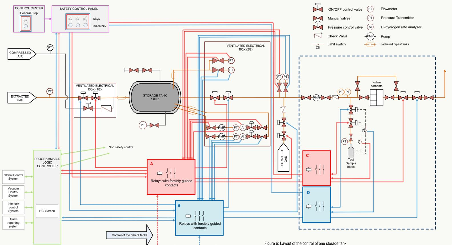
Figure 6: Layout of the control of one storage tank
