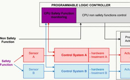
Figure 3: Safety control and non-safety control architecture
