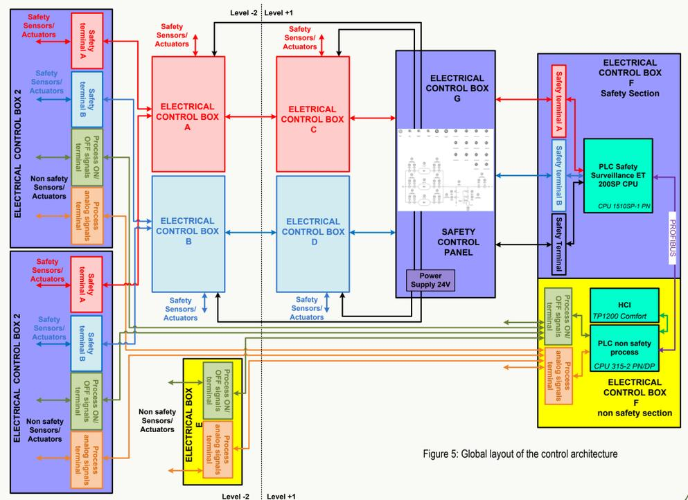
Figure 5: Global layout of the control architecture
