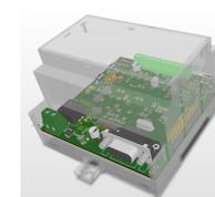
The terminal unit was designed to be installed inside the access booth known as Personnel Access Device (PAD). Thus, it is powered from a common 24V DC supply voltage rail of the PAD and connected to its controller via Profibus [9] as a Decentralised Peripheral (DP) slave device [10].
