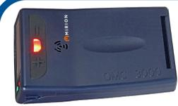
Operational dosimeters are provided by the Dosimetry Service at CERN. They are mandatory for everyone working in Limited Stay, High Radiation and Controlled Radiation areas [1]. The dosimeter displays the amount of dose and it has alarm functions when thresholds for dose or dose rates are exceeded. Before entering a hazardous area, the person has to read out and reset the dosimeter via a contactless reader terminal from the same manufacturer.
