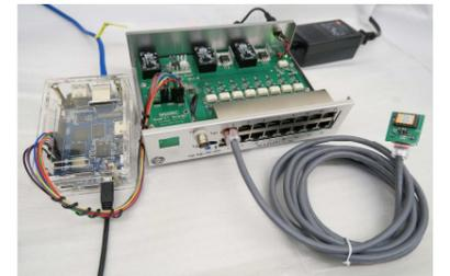
(b) Photo of the prototype 16 channels RadFET reader with BPI EPICS IOC.
