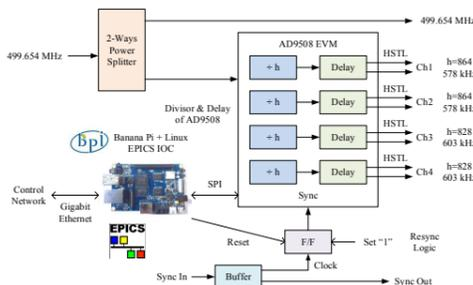
(a) Block diagram of programmable clock generator.
