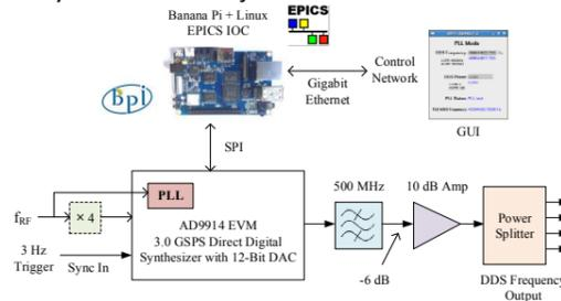
(a) Block diagram of the DDS control.
