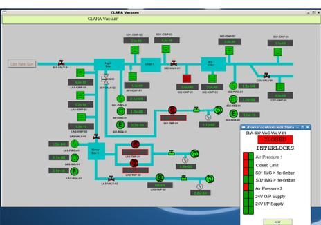
The status & interlocking system is responsible for on/off control and interlocking of hardware on the facility. It provides slow (>10ms) machine protection for technical sub-systems by only allowing operation of devices when predetermined conditions are met. It comprises of Omron CJ2M PLCs with digital I/O modules to marshal signals to and from hardware. ADC modules are also used to allow analog levels to produce interlocks directly within the PLC.
