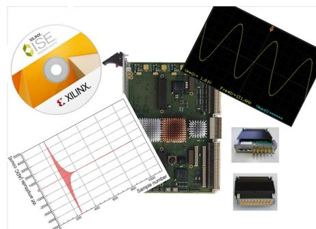
Stripline BPMs are digitised by a VME based system originally developed for EMMA. The system has been migrated from the MVME5500/vxWorks architecture of EMMA to the IOxOS IFC1210/Linux architecture for compatibility with the timing system. Diagnostic signals from cavity BPMs, bunch charge monitors, laser power meters and beam loss detectors will be sampled via systems using FMC data acquisition cards mounted on VME IFC1210 boards running EPICS.
