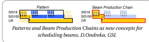
FAIR operation poses unique challenges with up to five parallel beams and pulse-to-pulse switching between particles. New parallel beam scheduling concepts have been designed and are now realized also in LSA, with first successful use at CRYRING.
