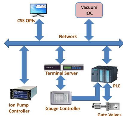
Figure 1: Vacuum Control Architecture
