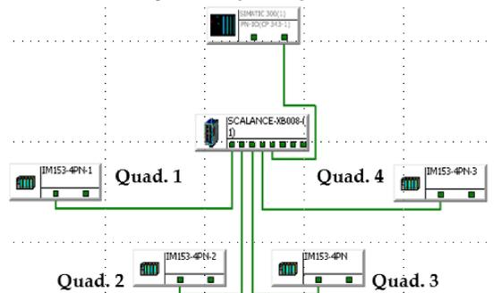
Figure 6: MPS PROFINET Architecture
