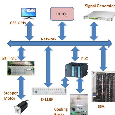
Figure 3: RF Control Architecture
