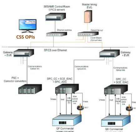
Figure 2: Power Supplies Control Architecture
