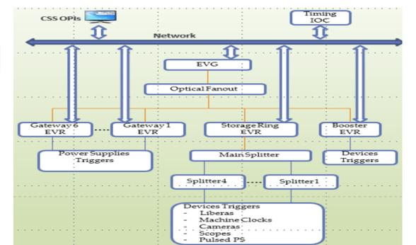
Figure 8: Timing Control System
