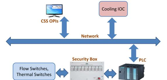
Figure 5: Cooling Control Architecture
