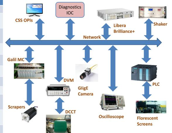
Figure 4: Diagnostics Control Architecture
