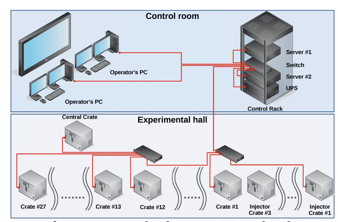
The system infrastructure is built upon COTS hardware: Intel x86-64 servers and multi-monitor x86-64 client machines.
