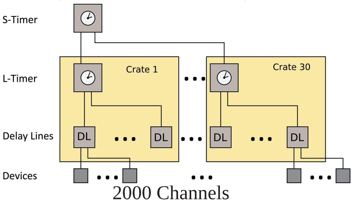
The synchronization subsystem provides all the controlled and controlling devices with the start pulses. The overall accuracy must be better than 4 ns across 70 m of length. This means that the propagation delays between the control units must be taken into consideration and negated.
