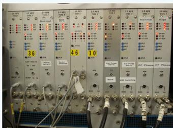
The original GP MPX units. Timing (T) and analogue function generator (F) modules are shown here.
