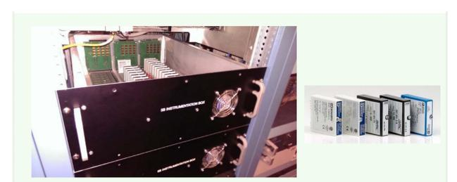
Figure 5: Instrumentation Box utilizing 5B Modules
