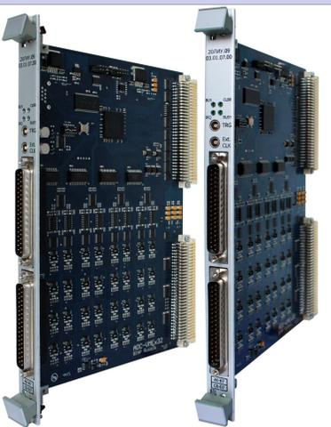
ADCx32 is the digitizer module that uses four 8 channel multiplexed 1 MSPS SAR ADCs with programmable channel sequencing. The sequence configuration determines sampling rate for each ADC channel individually.
