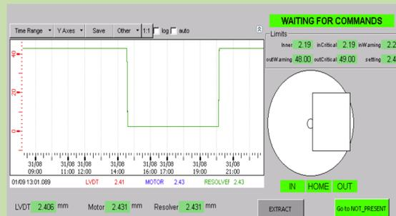
Part of the position FSM panel showing the pot position inside the beam pipe and a position plot
