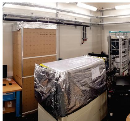
Figure 2: The system in a thermally stabilized environment; here with an insulated granite table, water circulation and system enclosure.
