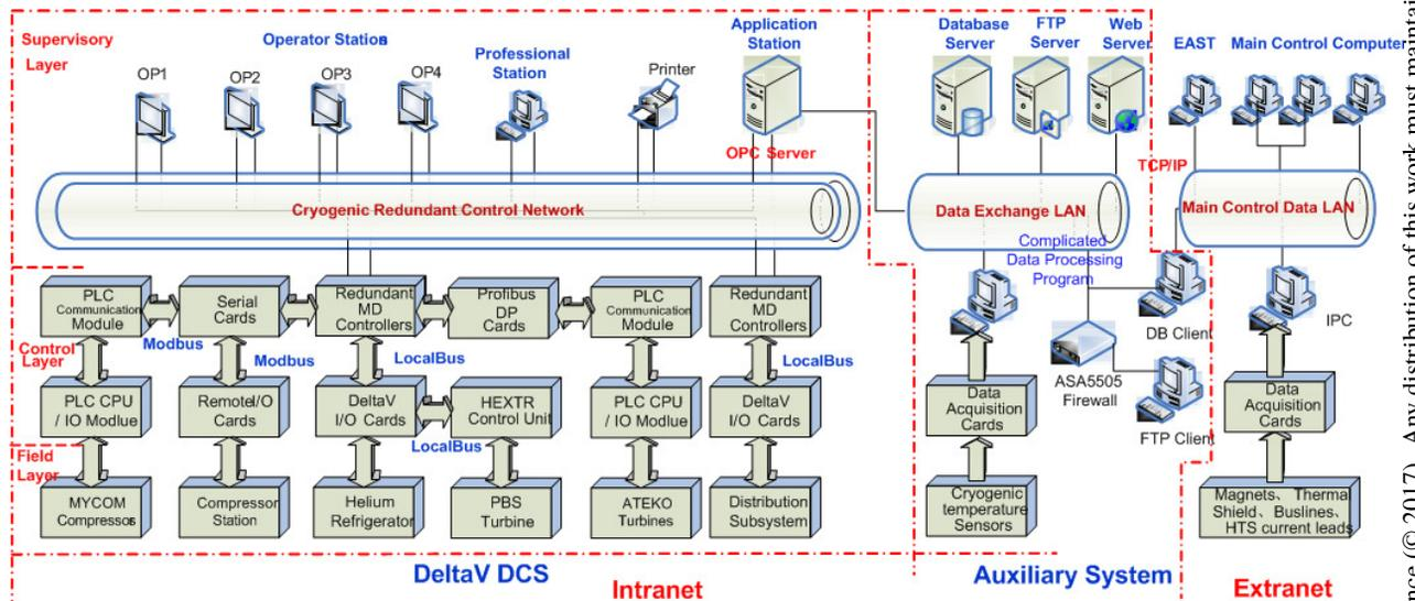
Figure 2: EAST cryogenic control system based on DelatV DCS.
