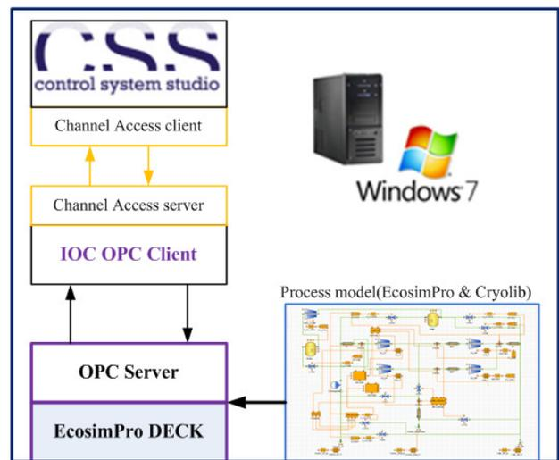
Figure 3: architecture of cryogenic process and control simulation.
