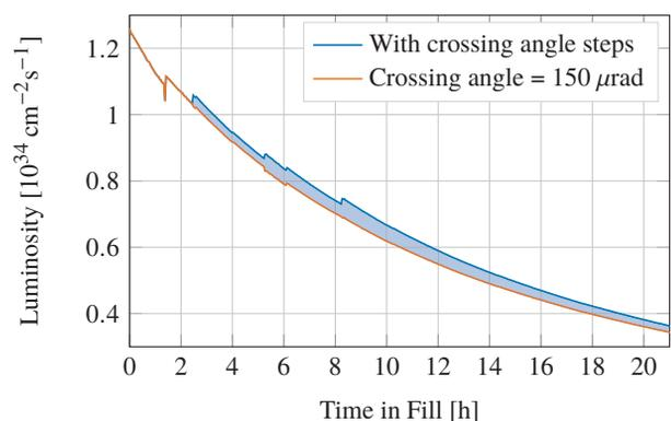
Figure 10: Luminosity evolution with crossing angle anti-levelling (LHC fill 5849). The gain in integrated luminosity (shaded area) is  $\sim 4\%$ .
