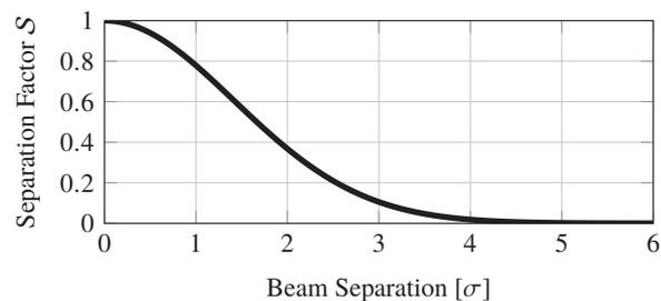
Figure 1: Separation factor as a function of the beam separation (in units of the beam size  $\sigma$ ).
