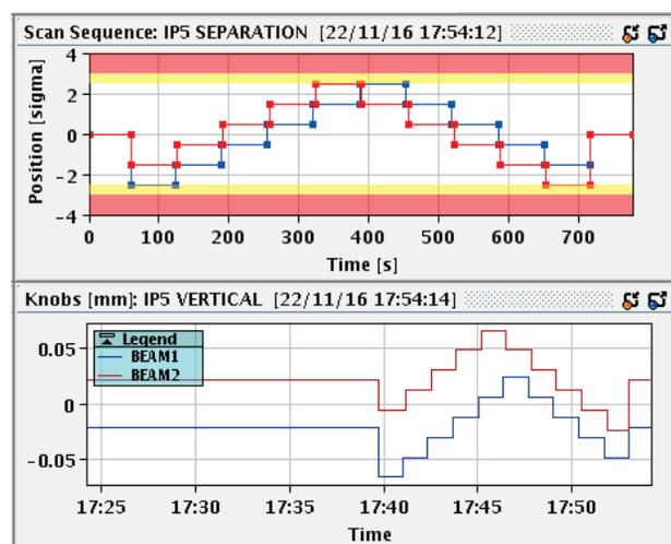
Figure 6: The CMS length-scale calibration scan run during the 2016 luminosity calibration session. The top panel shows the sequence as read from the file. The bottom panel shows the beam displacements sent to the control system while running the scan (the zero position is arbitrary).
