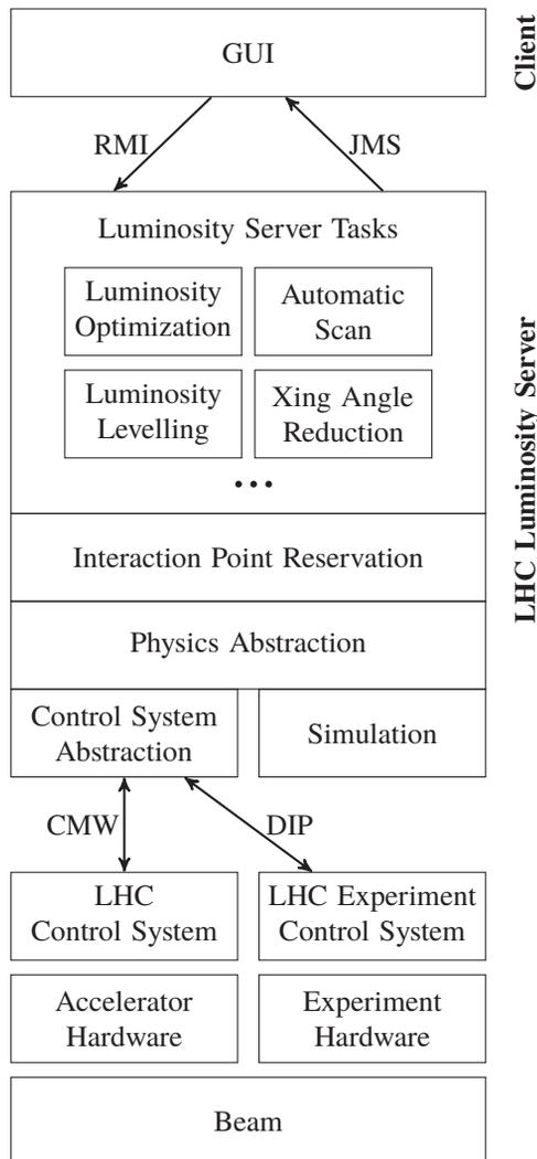
Figure 2: The new LHC luminosity software stack.
