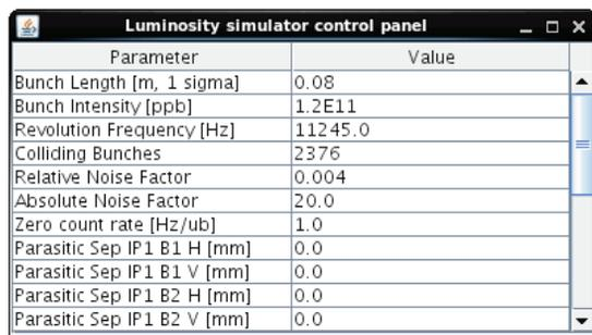
Figure 4: The control panel of the luminosity simulation loop of the LHC Luminosity Server. Any beam displacements that would be done are taken into account for the simulation.
