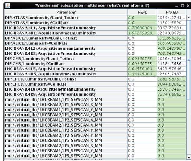
Figure 5: The subscription data source selector of the LHC Luminosity Server running in *wonderland mode*. At runtime, every subscription can be switched between the real acquisition and the internal simulation loop.
