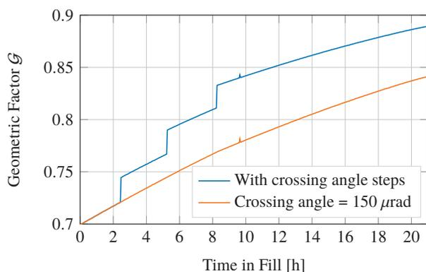
Figure 9: Evolution of the geometric factor  $\mathcal{G}$  with crossing angle anti-levelling (LHC fill 5849). At each step, the crossing angle was reduced by  $10 \mu\text{rad}$ .
