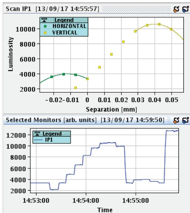
Figure 7: An example luminosity optimization in IP1. The top panel shows the acquired data points and fits. The bottom panel displays the raw luminosity signal; note the increase after applying the corrections.
