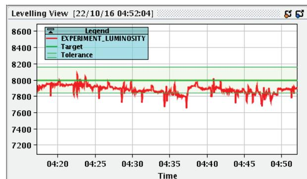
Figure 8: An example separation levelling status. At ~04:37 and at ~04:50, the beam separation was adjusted to bring the luminosity back into the target band.
