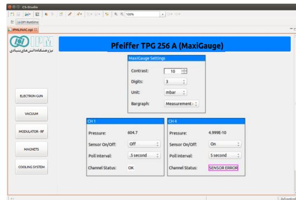
Figure 3: Vacuum setting operator screen.
