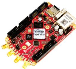
Figure 4: Red Pitaya board photograph, two analogue input and output pairs are visible on the left, LAN port, SD card with operating system and firmware on the right. [3]
