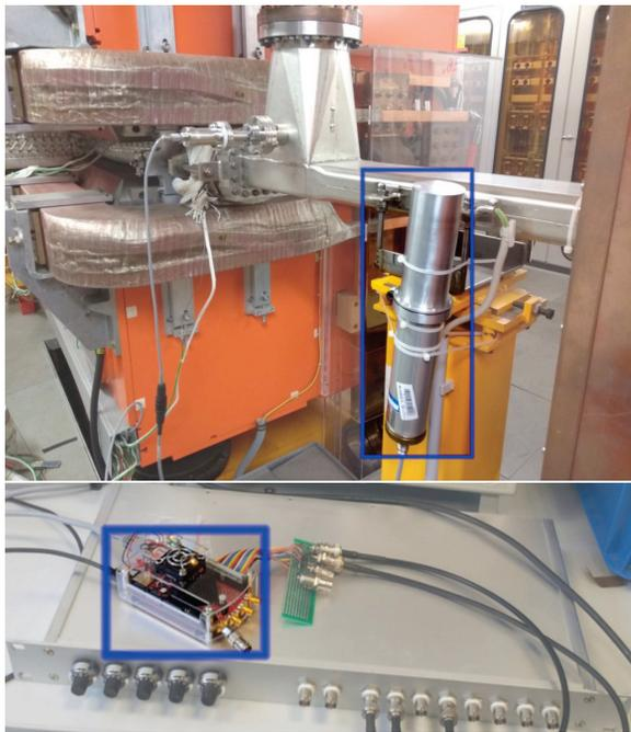
Figure 3: BLM hardware: the upper picture highlights one installed detector with scintillator and photomultiplier tube inside; the lower picture highlights the Red Pitaya board on top of a custom made discriminator module (usually housing a single Red Pitaya).
