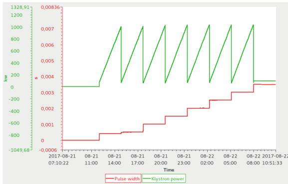
Figure 7: Complete RF Conditioning sequence data.
