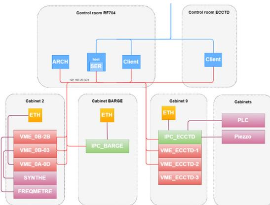
Figure 10: Network scheme of the Platform 704 MHz.
