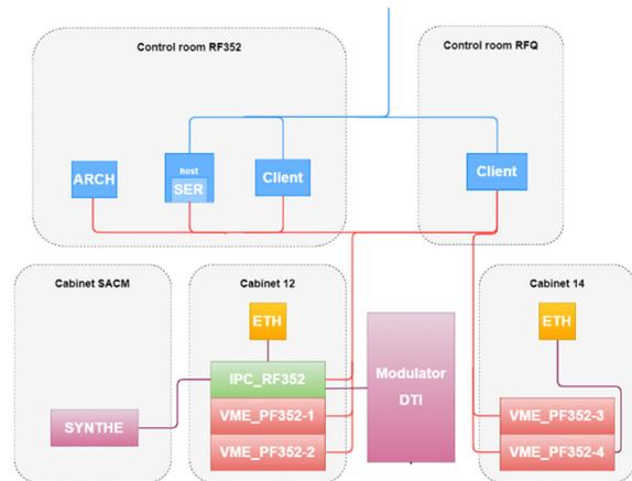
Figure 11: Network scheme of the platform 352 MHz.
