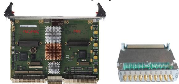
Figure 2: IOxOS cards (IFC1210 and ADC3111).
