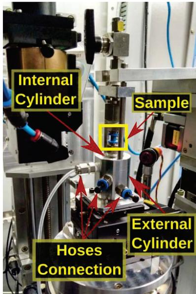
Figure 10: Flux cell mounted under IMX rotational stage.
