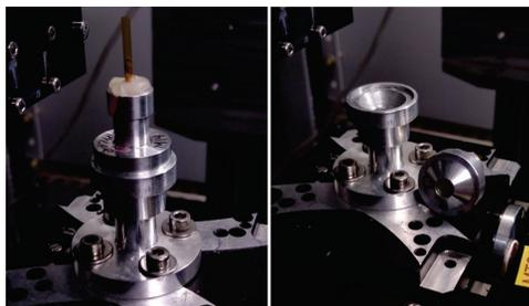
Figure 2: Conical sample holder.
