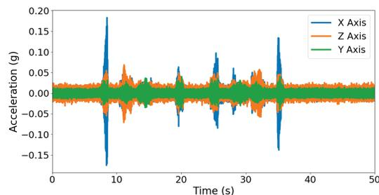
Figure 5: Sample point vibration caused by robot movement with 100% velocity and taking sample from the odd side of the tray.
