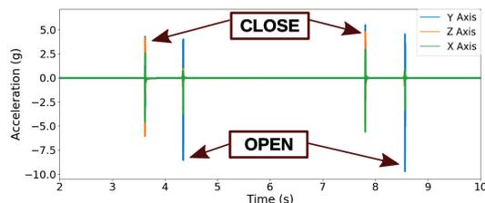
Figure 6: Vibration caused by opening and closing robot tool 5.15  $\mu$ m
