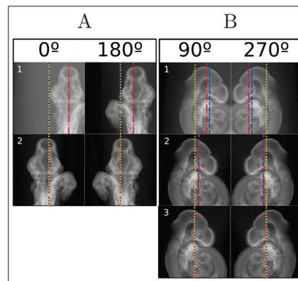
Figure 7: Iterations for sample alignment. In yellow is the centre of detector, blue is the axis of rotation and red is the centre of the sample.
