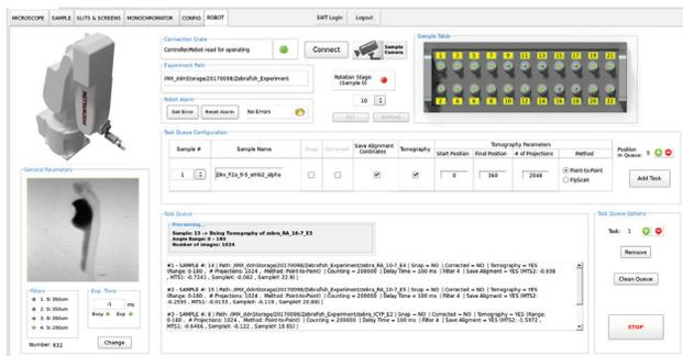
Figure 8: Graphical user interface for automatic system control.
