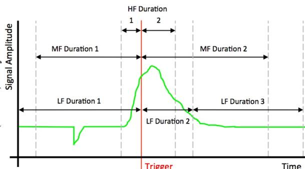
Figure 2: The timeline of a magnet recorded event.
