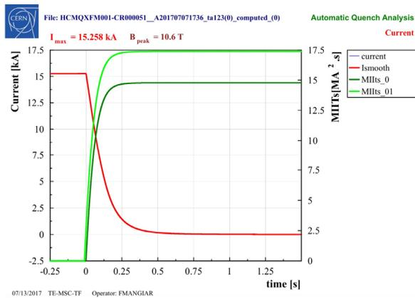
Figure 5: First quench of the MQXFS-5 magnet.
