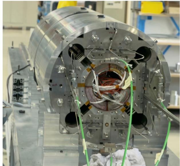
Figure 1: The assembly of the first model of the MQXFS quadrupole magnet.
