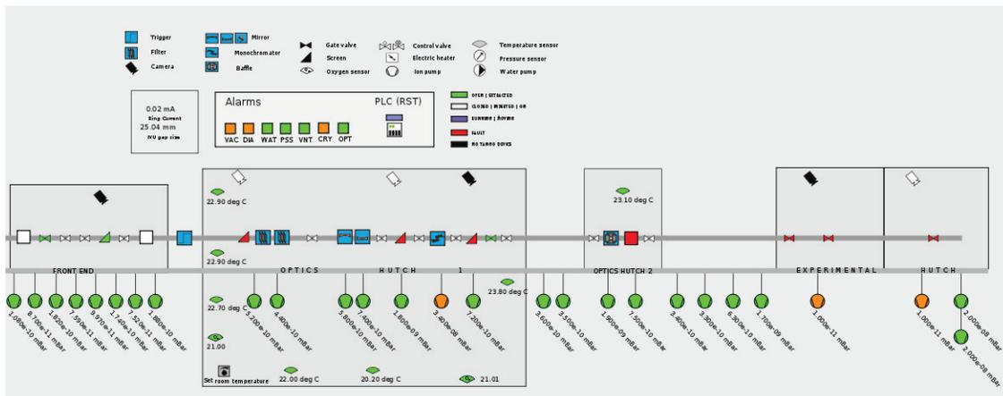
Figure 2: The Nanomax beamline as represented in the synoptic application. The coloured icons correspond to TANGO devices representing vacuum, diagnostic and optical elements, with the colour reflecting the value of the TANGO state.
