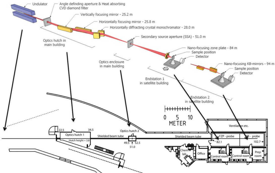
Figure 1: Overview of the Nanomax beamline showing the long optics section and the two end-stations.
