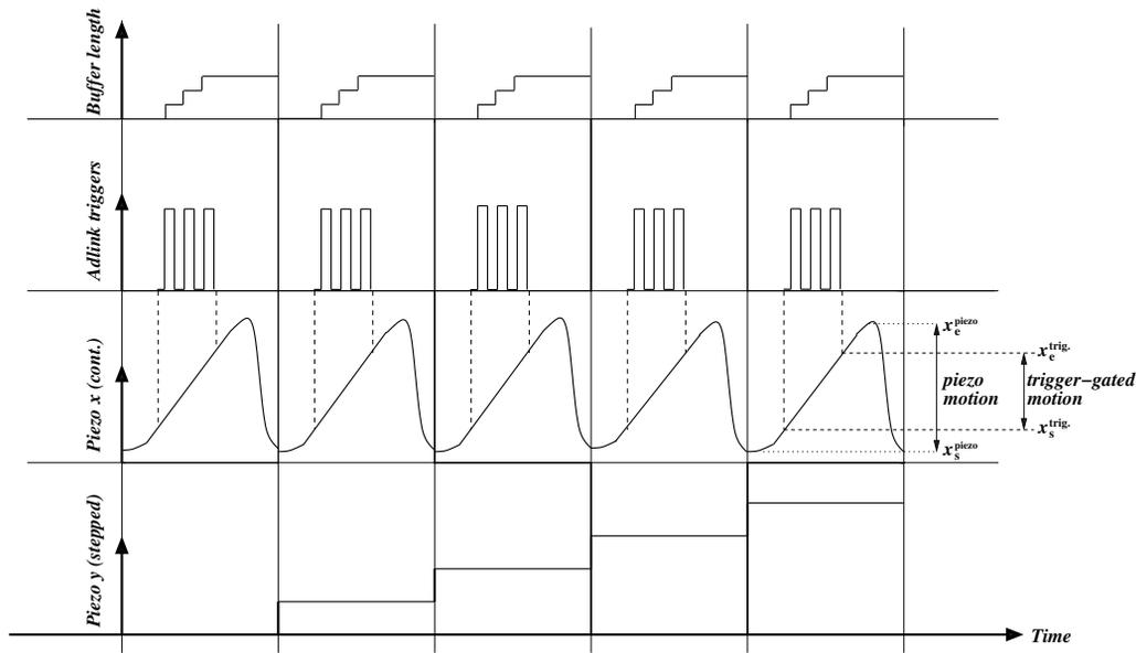
Figure 3: Generation of the time-based triggers by the Adlink 2005 card within the trigger-gated portion of the motion of the piezo  $x$  axis. In this example, three triggers are sent so the analogue input of the Adlink card also buffers three position measurements. After each continuous motion in  $x$  the buffer is read-out and the piezo is stepped in  $y$ .
